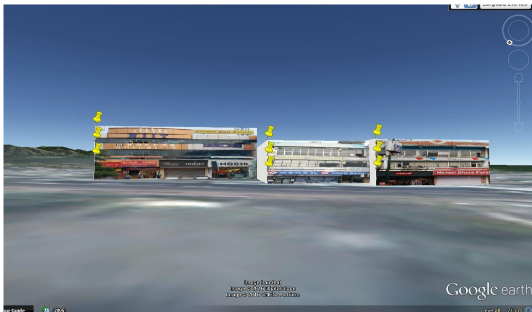
Fig 5.13: 3D view of point cloud near Madhuban, Rajpur Road using Nikon D60
